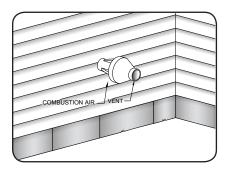
Note: See installation manual for proper dimensions & clearances of exhaust and air intake pipes and concentric terminations.
