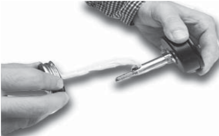
Figure 7 - Apply Pipe Sealant On Shaft of Gauge
