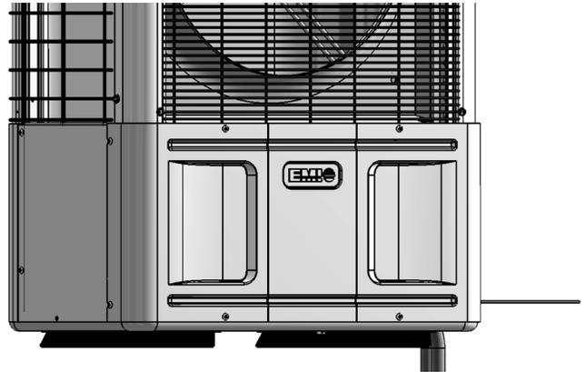
2. Remove the screws on the front of the panel.
