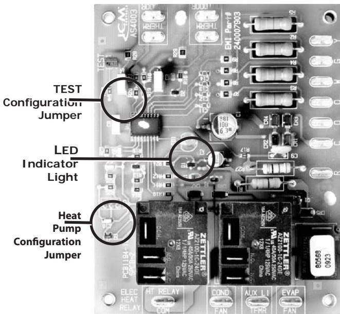
Two configuration jumpers are located on board, see Figure 8. Heat Pump Configuration Jumper is 3 pin jumper.
