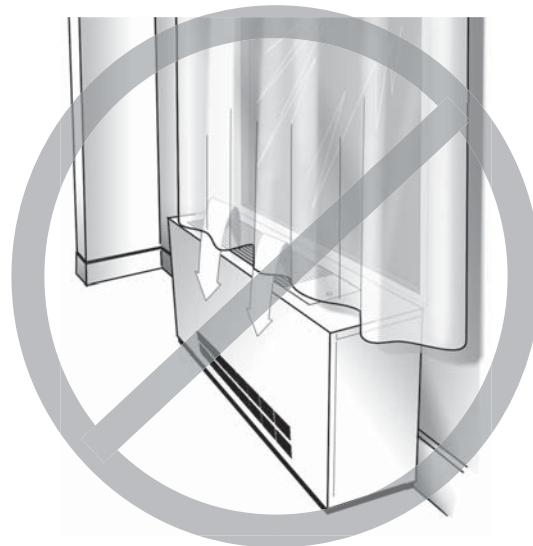
Figure 10 Restricted air flow diagram
