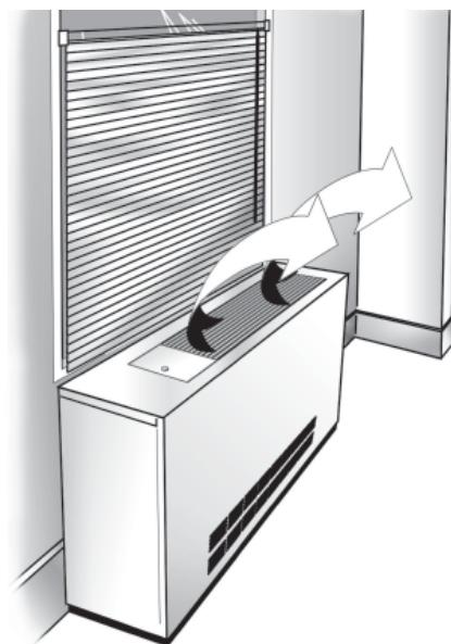
Figure 9 Proper air flow diagram
