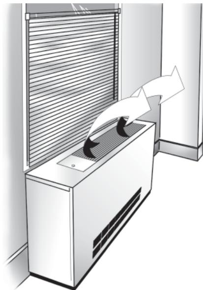
To ensure optimum performance of your PTAC/PTHP, avoid restricting the air flow. The position of curtains or drapes over supply air grille may cause air to recirculate without cooling the room. The unit will short cycle and may cause premature compressor failure (see Figure 8).
