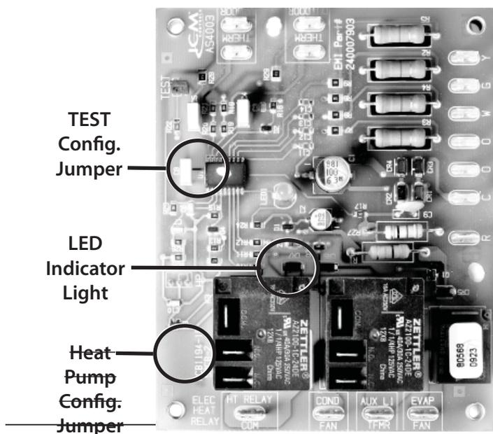
**Two configuration jumpers are located on the board, see Figure 8. The Heat Pump Configuration Jumper is a 3 pin jumper.**
