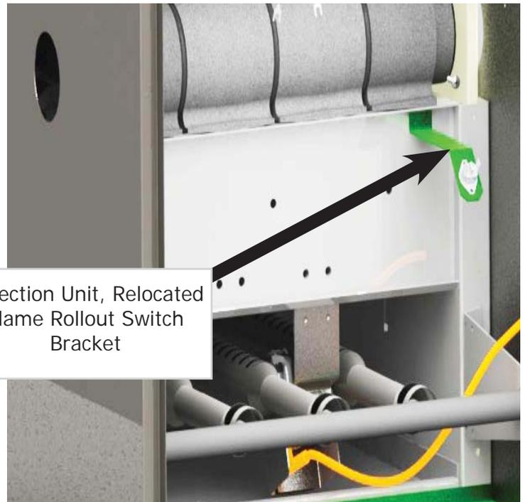
4 Section Unit, Relocated Flame Rollout Switch Bracket
