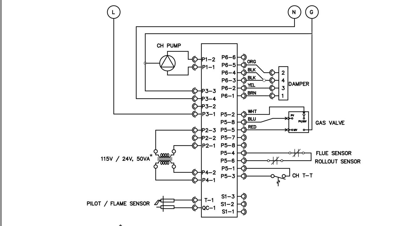
\* TRANSFORMER IS NOT SIZED TO ACCOMODATE VA REQUIREMENTS OF ZONE VALVES OR SIMILAR ACCESSORIES.
