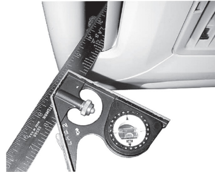
Figure 22 - Adjust Louver Position 30° From Plumb
