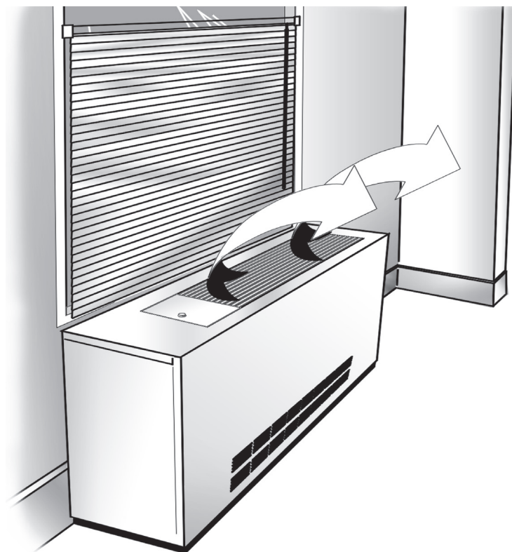
Figure 14 - Proper Air Flow Example
