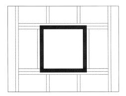
3. Insert downflow floor base in the floor opening with four (4) 9-1/2" wide tabs facing down. Tabs ensure 2" minimum clearance between combustible floor and supply air plenum. See Figure 2.
