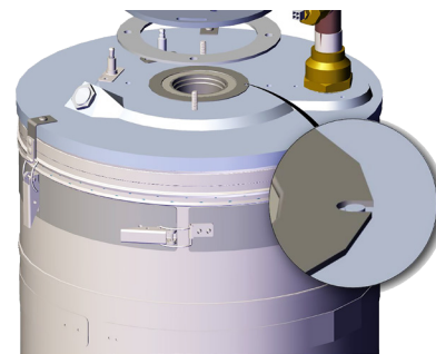
Figure 7 - Heat Exchanger Notch and Pin
