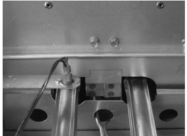
Figure 7 - Series 2 Final Pilot Tubing Configuration (2 Section Shown)
