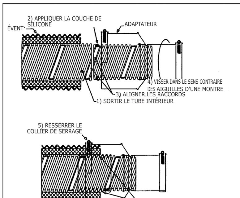
**Figure 11 : COMPOSANTS DU SYSTÈME D'ÉVACUATION Z-FLEX/GUIDE D'APPARIEMENT**
