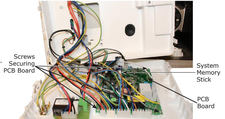
**Figure 4 - System Memory Stick Bevel**
