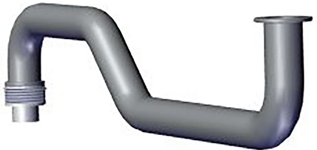
Figure 2 - Gas Pipe Removed - Nuts at each end not shown
