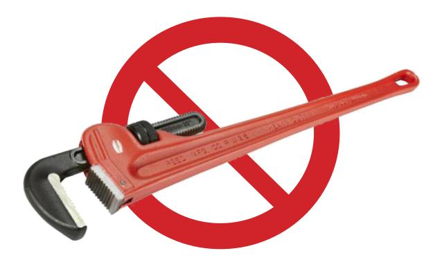
Use of a pipe wrench when making connections to boiler is not recommeded. Over tightening <u>WILL</u> result in water leaks.
