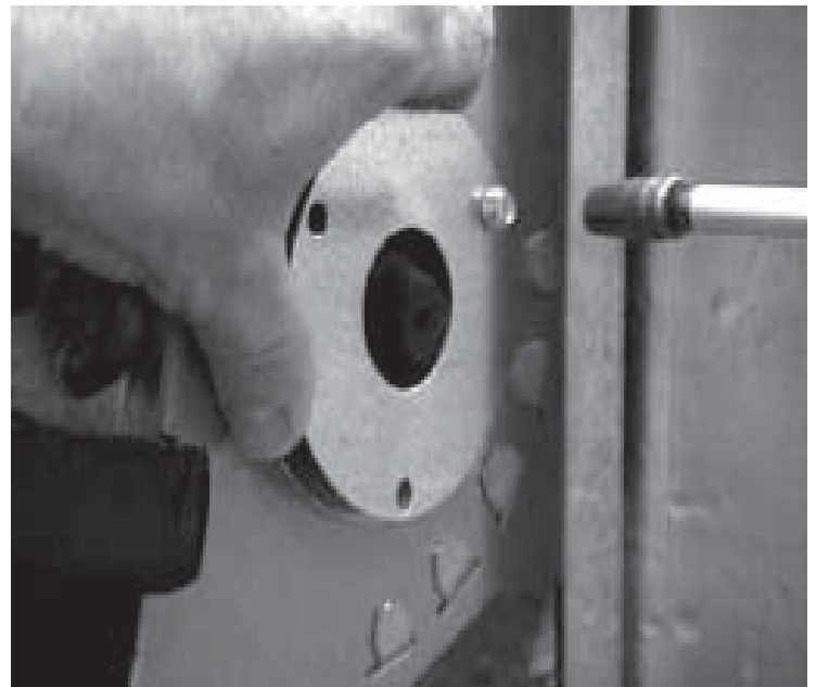
Figure 11 - Add Retainer Ring to Bearing
