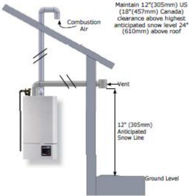
Sidewall vent w/ combustion air on roof
