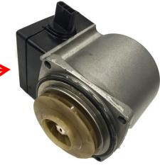
Pump motor removed from housing. Be sure gasket comes out with bad motor or remove from housing. Make sure new motor has new gasket in place before installing.
