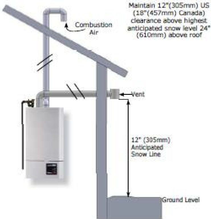
Sidewall vent w/ combustion air on roof
